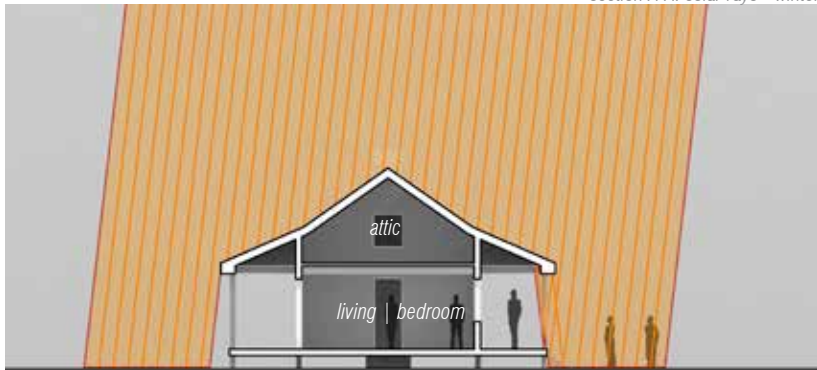
section A-A: solar rays - summer
