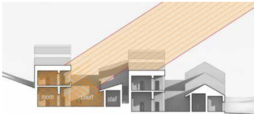
section A-A: solar rays - winter
