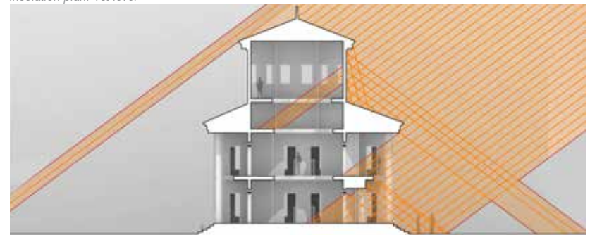
section A-A: solar rays - winter
