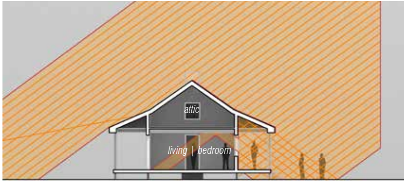
section A-A: solar rays - winter
