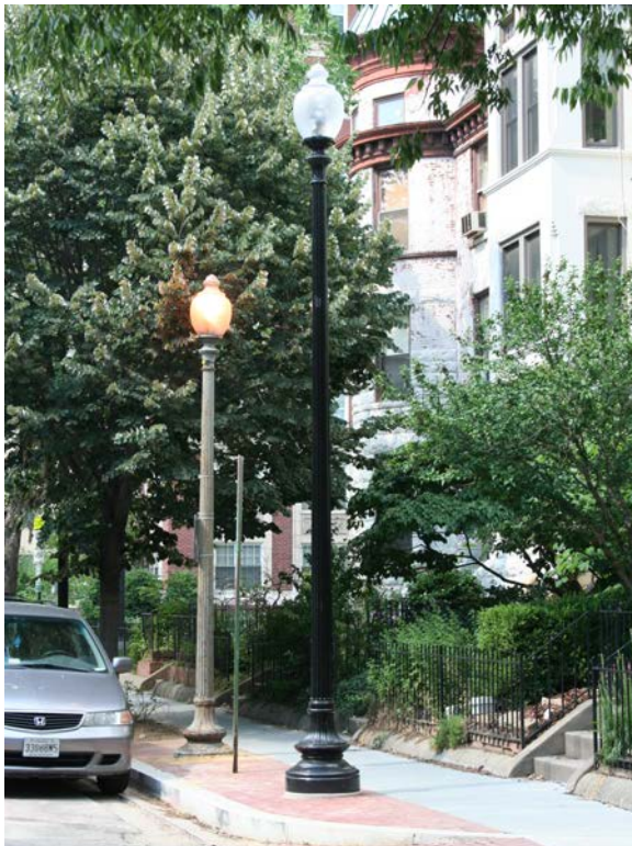
Washington, DC has been replacing historic light fixtures with near identical new lamps. However, the new lights, due to increased height, are having a negative impact on neighborhood scale. Paul Daniel Marriott
